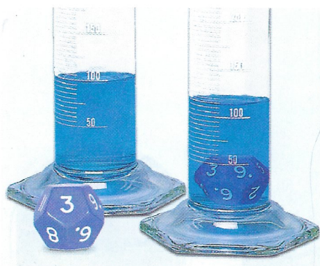
Figure 4 The 12-sided object displaced 15 mL of water. Because 1 \text{ mL} = 1 \text{ cm}^3 , the volume of the object is 15 \text{ cm}^3 .
