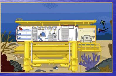
Underwater Research Station -Aguarius – underwater research and residential facility located in the Florida Keys. This underwater lab is located approx. 60 feet underwater and allows researchers to stay at this depth for days or weeks without surfacing (eating, sleeping, laboratory work, etc. everything is done here (think of it like an airtight Winnebago!) Read more about Aquarius at http://www.uncw.edu/aquarius
