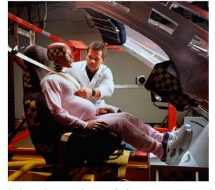
Some of the effects are obvious. In a crash, people in cars are exposed to physical force and as a result they usually get tossed around. That's obvious. Crash testing studies the forces car occupants are exposed to during a crash in a controlled, measurable environment. The data crash tests gather is so precise, it can help develop new and better safety systems.
