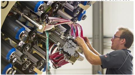
This high-tech contraption is known as an automated fiber placement, or AFP, machine. It has a round robotic head, with many spools of half-inch carbon-fiber ribbon attached to it. It can move around any shape exactly. Photo: Seattle Times/Mike Siegel
