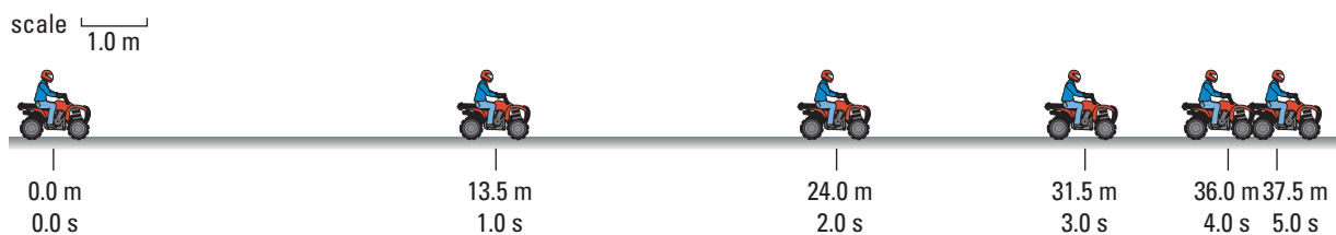
Figure 2.7 This ATV is undergoing non-uniform motion. It is accelerating, in this case, slowing down.
