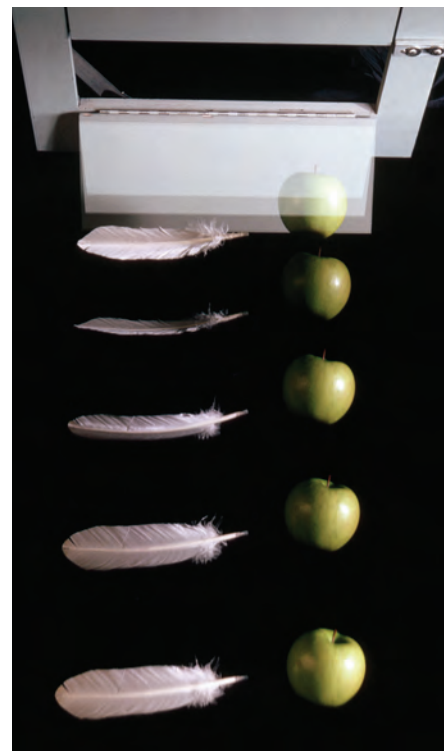
Figure 3.4 A demonstration with multi-flash photography: an apple and a feather are released simultaneously through a trap door in a large vacuum chamber and they fall together — almost. Because the chamber has partial vacuum, there is still some air resistance
