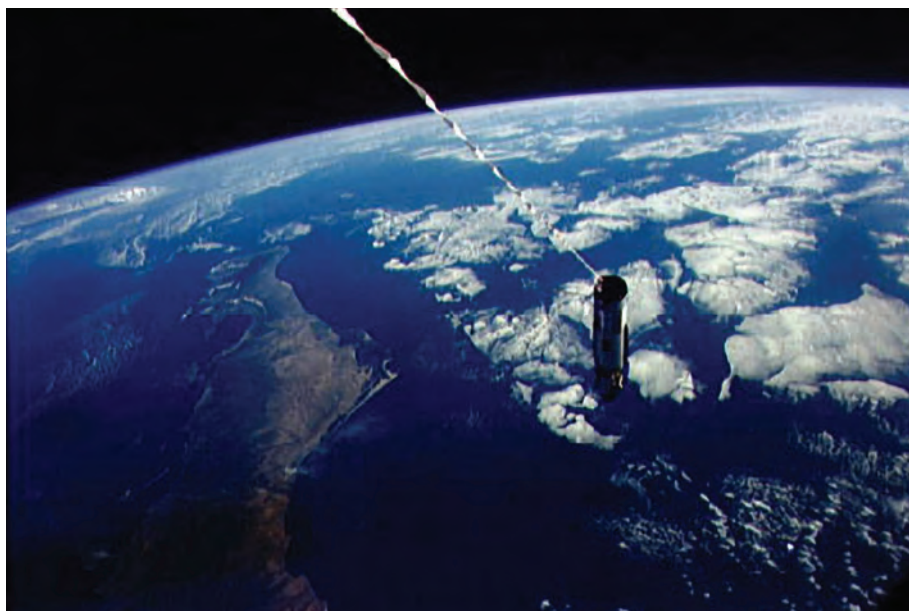
Figure 4.9 In this experiment, astronauts investigated whether a tether between their spacecraft (not shown) and a target spacecraft could be kept taut in orbit.
