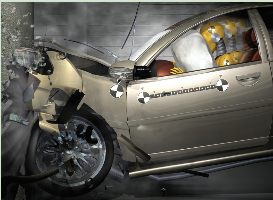
Figure 5.1 To design cars with better safety features, accident researchers use crash-test dummies to investigate the results of high-speed collisions.
