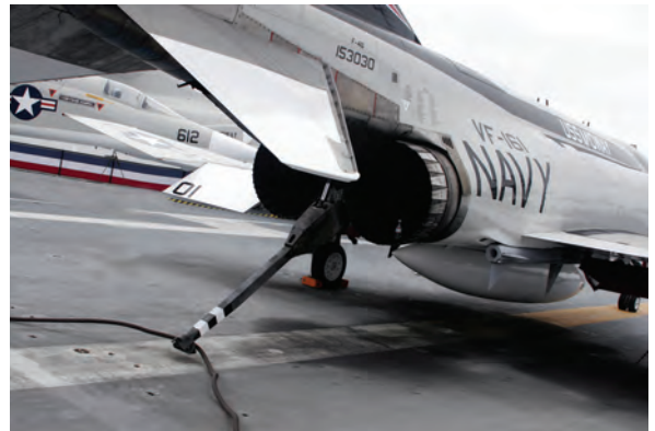
Figure 6.11 When the jet's tailhook catches the cable, kinetic energy is transferred from the jet, slowing it down.
