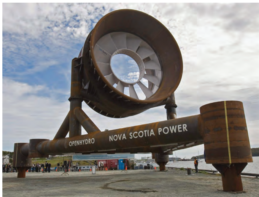
Figure 6.39 Each day, 100 billion tonnes of seawater flow in and out of the Bay of Fundy — more than the combined flow of the world's freshwater rivers. Underwater turbines like this one will soon generate up to 300 MW of electrical power — enough to power almost 100 000 homes.
