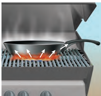
Figure 7.7 Radiant energy emitted by the burning coals in the barbecue heats the grill and the bottom of the pan. This energy is transferred to the rest of the pan by conduction. Thermal energy also passes from the grill to the pan to the food in the pan by conduction.
