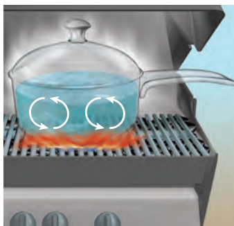
Figure 7.6 When you boil water, the water at the bottom of the pot is heated first, as thermal energy is transferred to the water from the pot by conduction. Convection in the water transfers energy through the movement of particles from one location to another.
