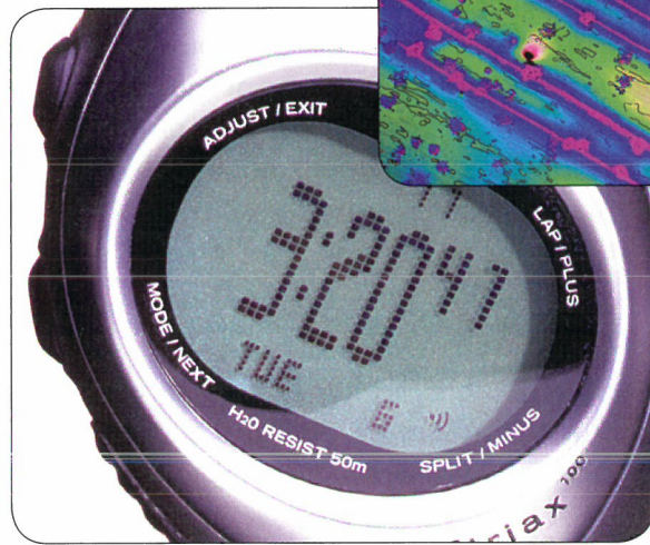
Digital watch displays are made possible through LCD technology. The inset photograph shows a polarized light micrograph of a LCD.
