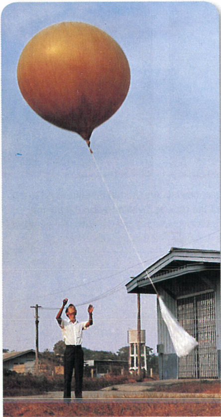
■ Figure 12.13 Radiosondes gather upper-level weather data such as air temperature, pressure, and humidity.
