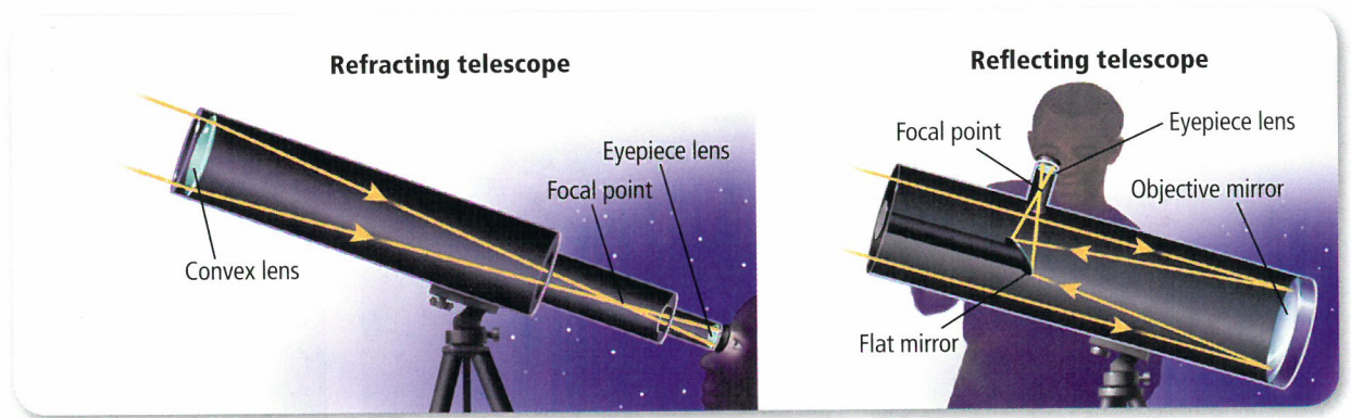
■ Figure 27.3 Refracting telescopes use a lens to collect light. Reflecting telescopes use a mirror to collect light.
