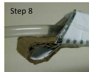
Now you should have an “arm” with a scoop on one end that you can open and close by manipulating the large syringe to move the scoop lid horizontally.
