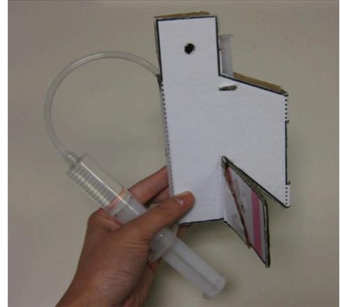
Now you should have a frame housing a syringe that will be responsible for lifting and dropping a mechanical arm, which you will be able to control using the larger syringe.
