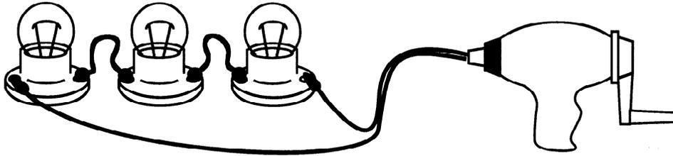
**Figure 4.** A hand-powered series circuit
