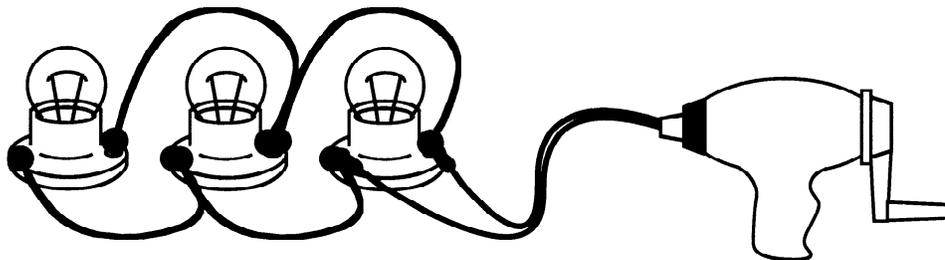
**Figure 5.** A hand-powered parallel circuit
