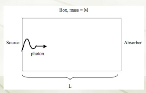
By conservation of momentum, when the photon leaves the source, and travels right, the box must move to the left to maintain a total momentum of 0 in the system. We will use two methods to calculate how far the box moves, and equate the results.
